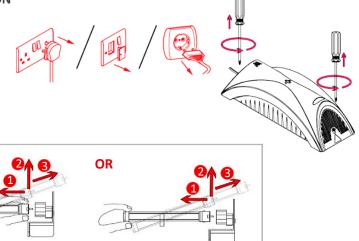
If you are fitting a NEW lamp, firmly grip lamp terminal/connector end (or end cap) and carefully slide lamp into the socket and spring clip.
